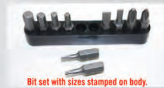
Bit set with sizes stamped on body.
